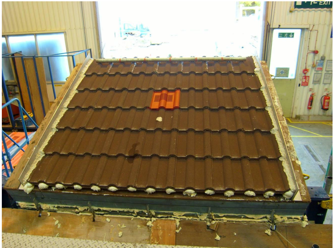
Figure 3 An general view of the roof tiles and the Manthorpe large format concrete interlocking tile vent installed in the test roof.
