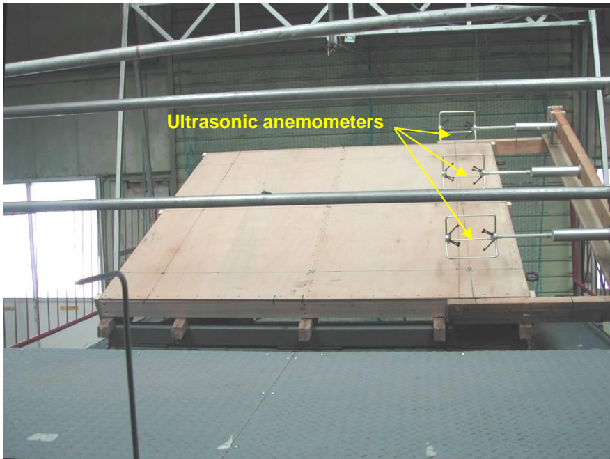
Figure C2 Calibration of the wind speed over the test specimen area
