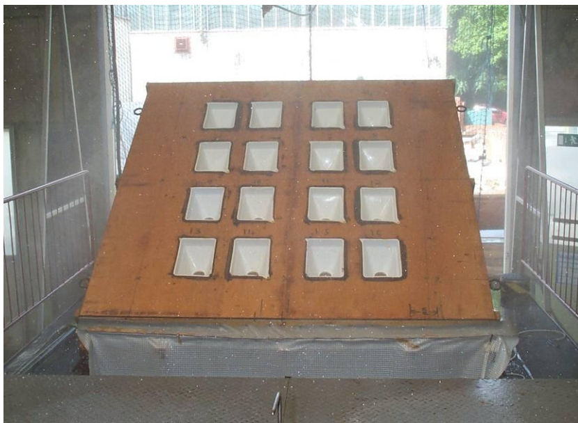
Figure C6 View of the 16 rainfall collection buckets on the test rig
