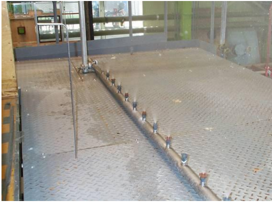
Figure C3 Bottom spray bar
