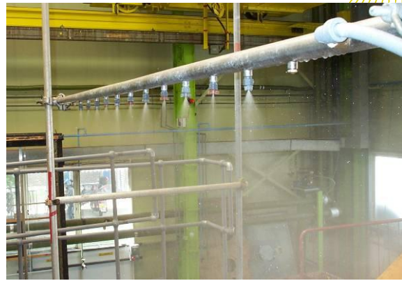
Figure C4 Top spray bar
